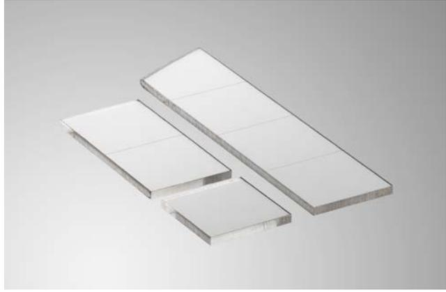
Single-pass (300 mm/s) dicing of 500  $\mu$ m thick 4H-SiC wafer.
