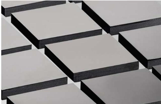
Precise dicing of a silicon wafer.
