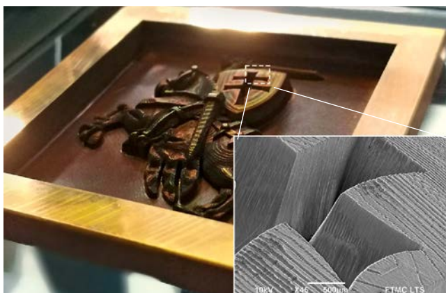
3D-milled sample in copper. Zoom-in SEM image.
