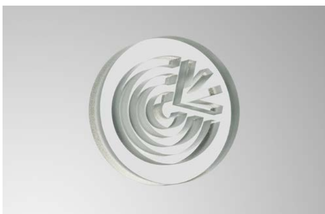
Structure fabricated in fused silica.
