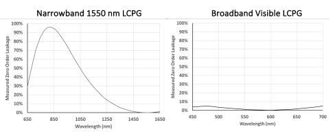
The plots above illustrate the typical diffraction spectra of narrowband (left) and broadband (right) LCPGs by measuring the leakage into the O<sup>th</sup> order (i.e., undiffracted transmission). Peak diffraction efficiency occurs where the plots have a null, representing >99.5% diffraction efficiency in both cases.
